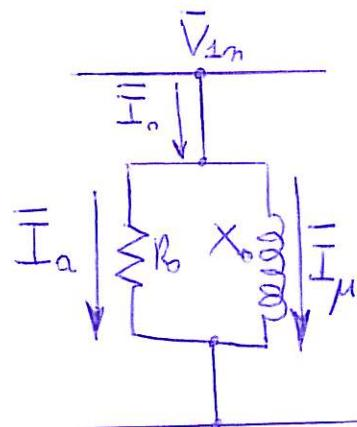
$$I_\mu = \frac{V_{1m}}{X_o}$$
