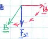
$$F_{SR} = \int_{x_0}^{x_0+a} i_b u_x \frac{\mu_0 i}{2\pi(y+a)} u_z dx$$
