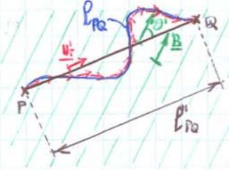
$$\underline{F}_{\text{m}} = I B \sin 90^\circ \underline{P.Q.} \underline{u}_r$$
