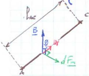
$$\underline{F}_{\text{m}} = \int_{\text{P}}^{\text{Q}} I \underline{u}_r \times \underline{B} d\underline{l} = \int_{\text{P}}^{\text{Q}} I B \sin 90^\circ \underline{u} d\underline{l} = \text{per } \underline{u}_r = \text{direzione costante} \\ \sin \theta = \text{cost.}; \underline{u} = \text{dir. cost.} \\ = I B \sin 90^\circ \int_{\text{P}}^{\text{Q}} d\underline{l} = \boxed{\underline{F}_{\text{m}} = I B \cdot \text{lung. P.Q.} \underline{u}}$$
