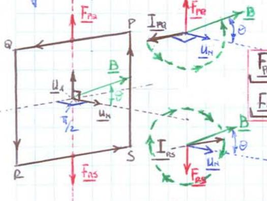
$$\underline{F}_{\text{PQ}} = I \overline{PQ} B \sin(90^\circ - \theta) \underline{u}_1 = I b B \cos \theta \underline{u}_1$$
