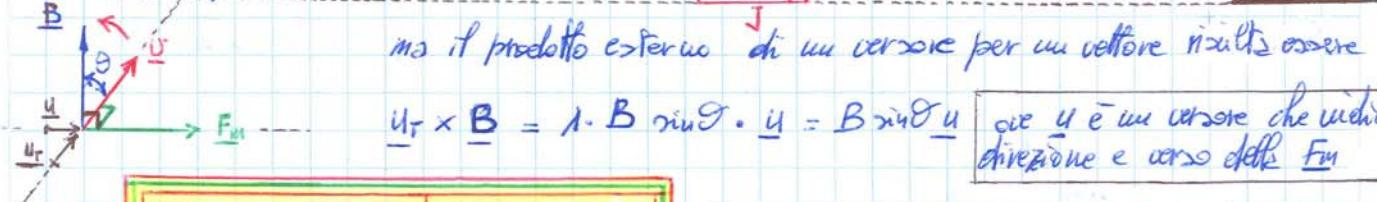
$$dF_m = IB \sin \theta \underline{U_r} \underline{v} = dF = I \underline{U_r} \times \underline{B} d\underline{l}$$
