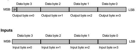
The preset adjustment value transferred in data bytes is accepted as position value with the leading edge of bit 32 (=bit 7 of data byte 3) or bit 16 (=bit 7 of data byte 1).
