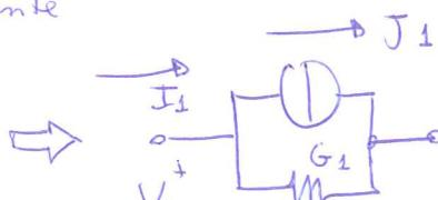
$$I_1 = J_1 + G_1 V_1 \quad \begin{cases} G_1 = \frac{1}{R_1} \\ J_1 = \frac{E_1}{R_1} \end{cases}$$
