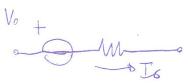
$$V_6 = E_6 + R_6 I_6$$
