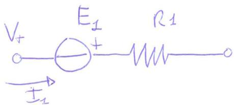
$$V_2 = -E_1 + R_1 I_1$$
