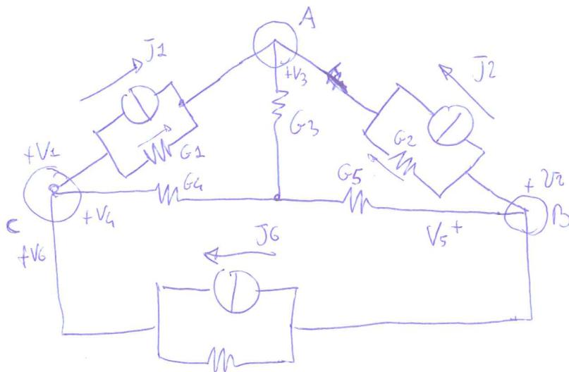
$$\left. \begin{array}{l} -G_1 V_1 - G_2 V_2 + G_3 V_3 = J_1 + J_2 \\ +G_2 V_2 + G_5 V_5 - G_6 V_6 = -J_2 - J_6 \\ +G_1 V_1 + G_4 V_4 + G_6 V_6 = -J_1 + J_6 \end{array} \right\} \sum \pm G_i V_i = \sum \pm J_i$$
