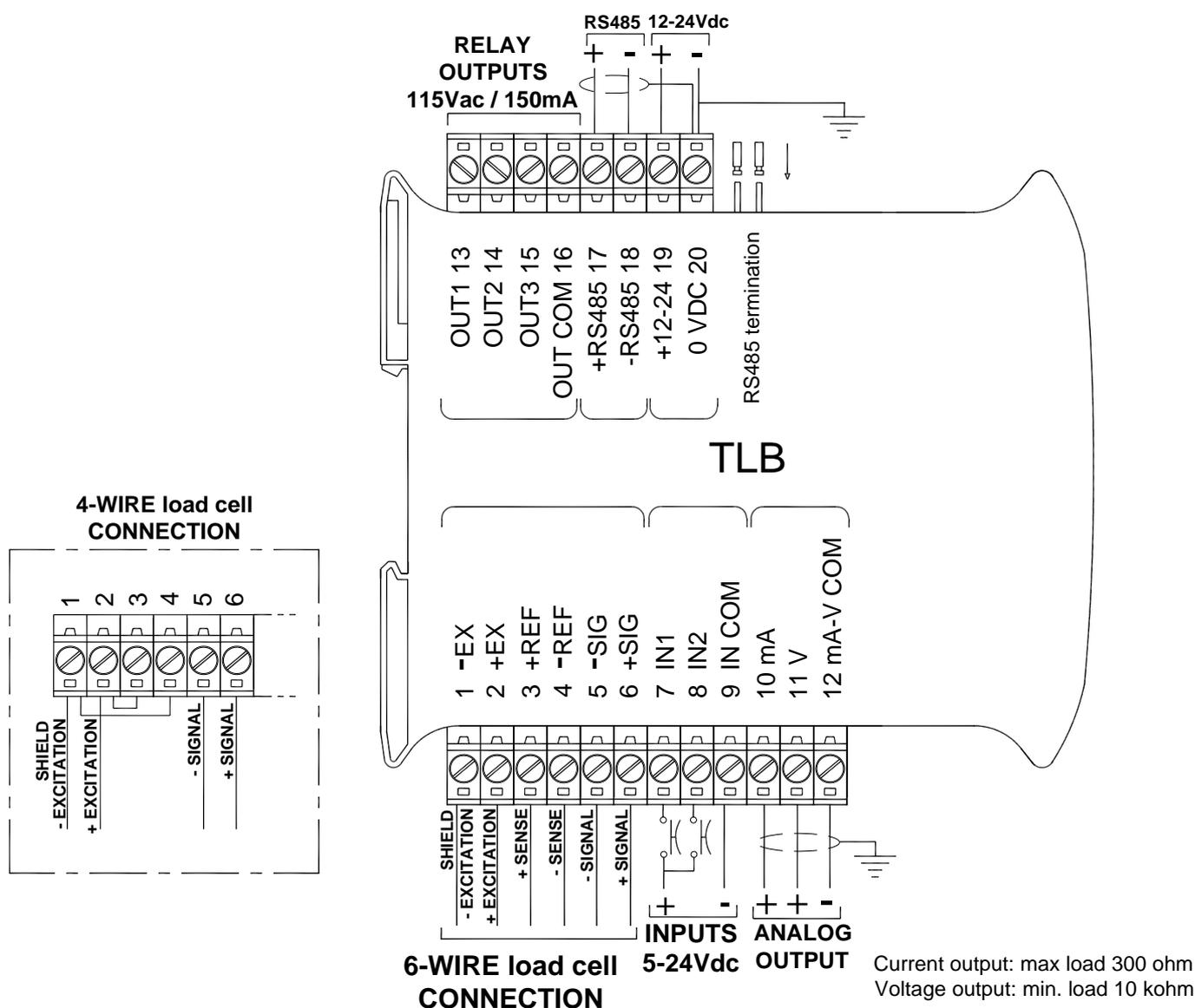
**3 outputs:** settable setpoints or remote output management via protocol.
