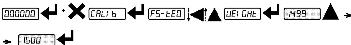
After having performed the THEORETICAL CALIBRATION and TARE WEIGHT ZERO SETTING, this function allows correct calibration to be done using sample weights of known value, if necessary, any deviations of the indicated value from the correct value to be corrected.
