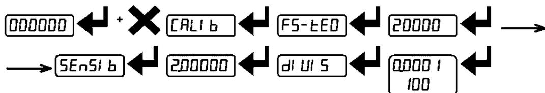
This function allows the load cell rated values to be set.
