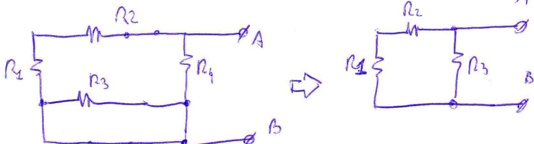
$$Reg_{AB} = \frac{R_2 + R_4 + R_1}{(R_1 + R_4 + R_2)} = \frac{40 + 40}{80} = 20 \Omega$$
