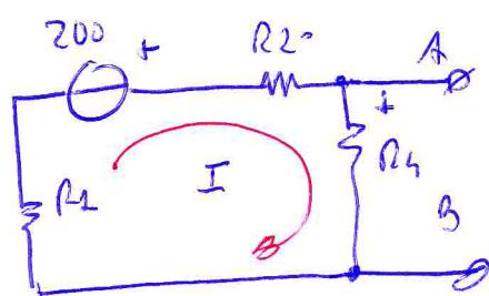
$$I = \frac{E_L}{R_2 + R_L + R_4} = \frac{200}{80} = 2.5 \text{ A}$$
