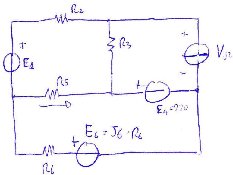
$$\left\{ \begin{array}{l} (R_2 + R_3 + R_5) i_2 - R_3 i_b - R_5 i_c = E_1 \\ R_3 i_b - R_3 i_a = E_1 - V_{J2} \\ (R_5 + R_6) i_c - R_5 i_a = -E_6 + V_{J2} \\ i_b = -J_2 \end{array} \right.$$
