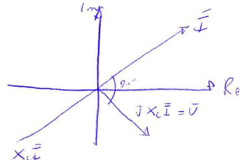
$$v(t) = V_m \sin(\omega t + \alpha) \quad i(t) = V_m \sin(\omega t + \alpha + \frac{\pi}{2})$$
