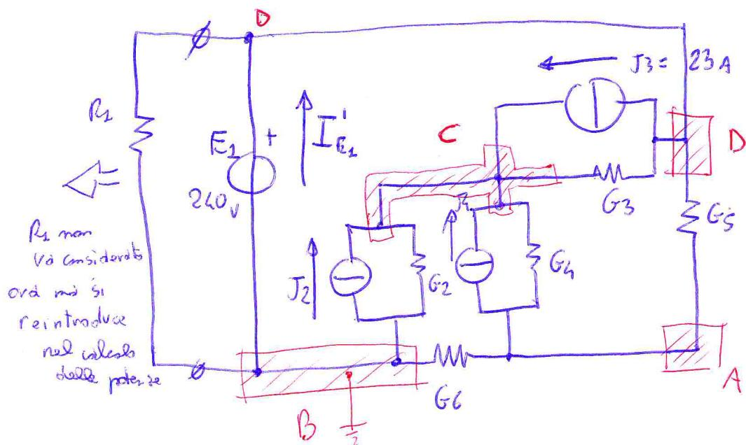
$$\left\{ \begin{array}{l} (G_4 + G_5 + G_6) V_A - G_5 V_D - G_4 V_C = -J_3 \\ (G_2 + G_5) V_D - G_3 V_C - G_5 V_A = -J_3 + I_{E_1}^1 \\ (G_3 + G_4 + G_2) V_C - V_D G_3 - V_A G_4 = +J_3 + J_2 \end{array} \right.$$
