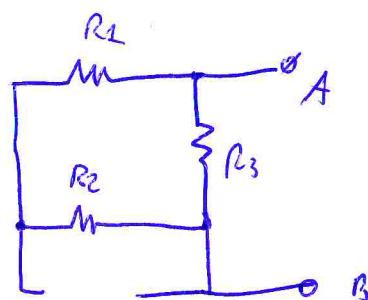
$$R_{eq\, Th} = \frac{(R_2 + R_3) \cdot R_3}{R_1 + R_2 + R_3} = 3 \Omega$$
