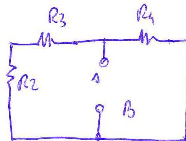
$$R_{AB} = R_4 / (R_2 + R_3) = 100 \Omega$$
