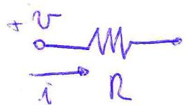
$$v(t) = V_m \sin(\omega t + \alpha) \quad i(t) = \frac{V_m}{R} \sin(\omega t + \alpha)$$
