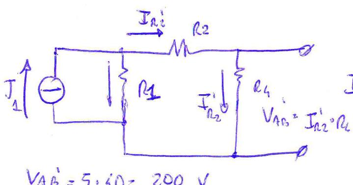
$$I_{AB} = \frac{J_2 \cdot R_4}{R_1 + (R_2 + R_4)} = \frac{20 \cdot 20}{20 + (20 + 40)} = \frac{400}{80} = 5A$$
