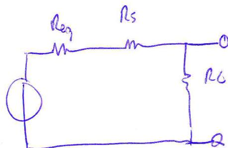
$$V_{AB} = \frac{E_{eq} \cdot R_L}{R_S + R_L + R_0} = \frac{90 \cdot 10}{12.5 + 17.5 + 10}$$
