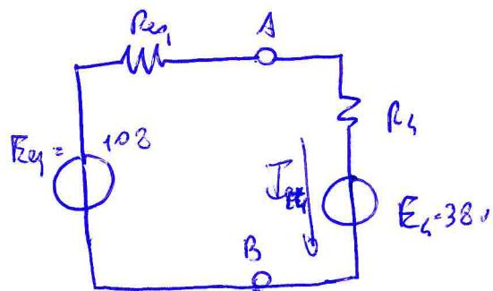
$$E_g - E_{g\text{eq}} + (R_g + R_4) \cdot I_{R_4} = 0$$
