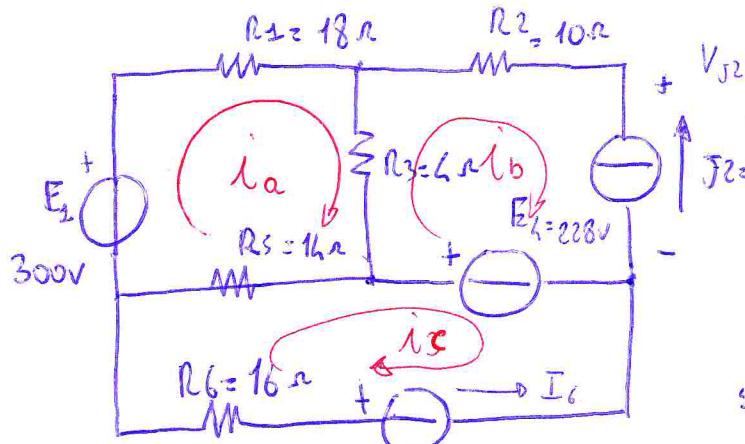
$$\begin{cases} i_a(R_1+R_3+R_5) - i_b(R_3) - i_c(R_5) = +E_1 \\ -i_a(R_3) + i_b(R_2+R_3) = -V_{J2} + E_6 \\ -i_a R_5 + i_c(R_5+R_6) = -E_6 + E_6 \end{cases}$$
