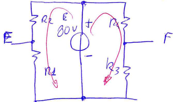
$$V_{R1} = \frac{E}{R_2 + r_s} \cdot R_1 = \frac{80}{20} \cdot 10 = \frac{800}{20} = 40 \text{ V}$$
