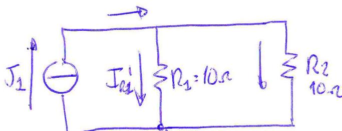
$$I_{R1}' = \frac{J_1}{R_1 + R_2} \cdot R_2 = 2A$$
