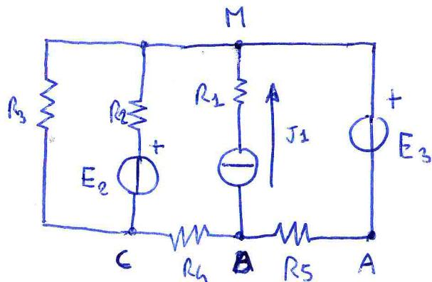
$$\begin{array}{ll} R_1 = 10 \Omega & J_1 = 4 A \\ R_2 = 6 \Omega & E_2 = 20 V \\ R_3 = 5 \Omega & E_3 = 40 V \\ R_4 = 10 \Omega & \end{array}$$
