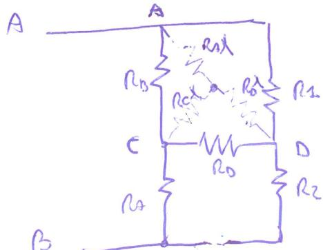
$$\left\{ \begin{array}{l} R_{A\lambda} = \frac{R_B \cdot R_1}{R_B + R_D + R_1} \\ R_{C\lambda} = \frac{R_B \cdot R_D}{R_B + R_D + R_1} \\ R_{D\lambda} = \frac{R_1 \cdot R_D}{R_B + R_D + R_1} \end{array} \right.$$
