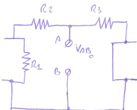
$$\text{Reg}_{AB} = \frac{(R_2 + R_1) \cdot R_3}{(R_2 + R_1) + R_3} = \frac{350}{45} = 7,77 \Omega$$
