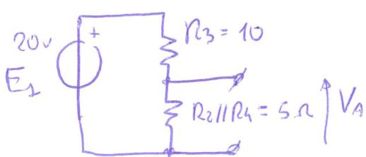
$$V_{A'} = \frac{E_1}{R_3 + (R_2 || R_3)} = \frac{20}{10 + 5} = 6,66 V$$
