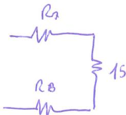
$$R_{eq_{tot}} = R_A + R_B + R_o = 50 + 15 + 50 = 115 \Omega$$
