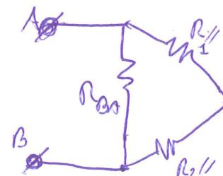
$$R_S = R_1// + R_2// = 214,287 \Omega$$
