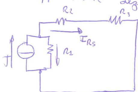
$$I_{RS} = \frac{J}{(R_2 + R_3) + R_1} \cdot R_1 = \frac{1 \cdot 25}{45} = 0,555 \text{ A}$$
