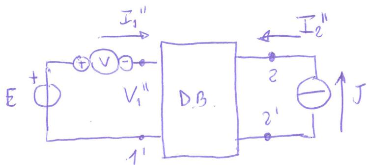
$$\left\{ \begin{array}{l} V_1'' = E - V_V = R_{11} I_1'' + R_{12} + I_2'' \\ V_2'' = R_{21} I_1'' + R_{22} I_2'' \end{array} \right. \quad \left. \begin{array}{l} \text{R.V.} \\ \text{AGGIUNTIVA} \end{array} \right\} \left\{ \begin{array}{l} I_1'' = 0 \\ I_2'' = J \end{array} \right.$$
