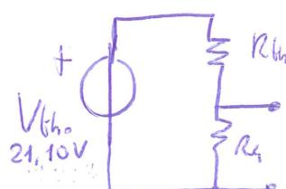
$$V_{RL} = \frac{V_{th}}{R_{th} + R_L} \cdot R_L$$
