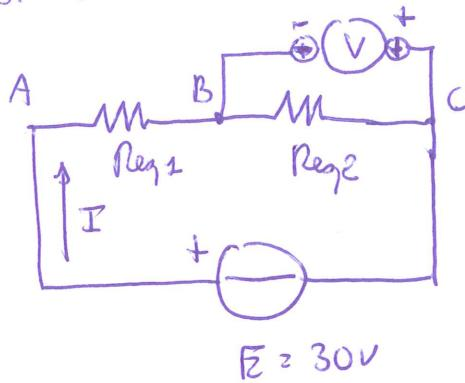
$$Reg_1 = (R_2 // R_3) + R_1 = 8 \Omega$$
